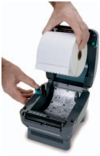
4. Make sure that the core is resting on the hangers and that the roll turns freely. The roll must not sit in the bottom of the media compartment.
