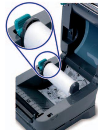
5. Close the printer cover. Connect the power cord to the printer first and then to the power source (e.g., wall outlet). Ensure that the labels are installed correctly.
