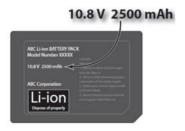
The calculation used to determine watt hours is: **Volts x ampere hour (Ah) = watt hours** Example: "10.8 V 2500 mAh" contains the information needed to determine the watt hours for this battery.
