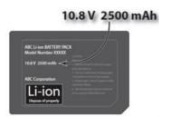
The calculation used to determine watt hours is: **Volts x ampere hour (Ah) = watt hours** Example: "10.8 V 2500 mAh" contains the information needed to determine the watt hours for this battery.
