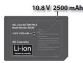
The calculation used to determine watt hours is: Volts x ampere hour (Ah) = watt hours Example: "10.8 V 2500 mAh" contains the information needed to determine the watt hours for this battery.
