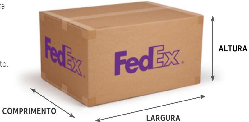
$$\text{Peso dimensional} = \frac{\text{COMPRIMENTO} \times \text{LARGURA} \times \text{ALTURA}}{5.000} = \text{Kg dimensionais}$$
