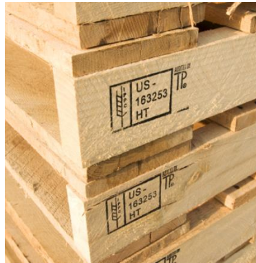
The IPPC mark the ISPM15 requires on treated wood packaging material
