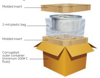
This design protects the rim from dents, scratches, and abrasions. The molded inserts are designed to fit multiple sizes.
