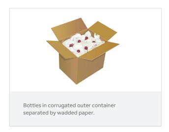
Paper dunnage can compress under internal movement of contents and allow glass containers to become unstable.
