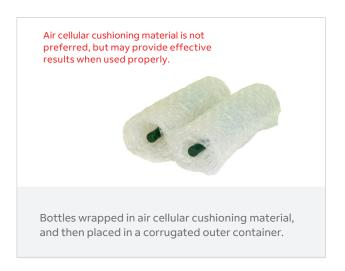
Air cellular cushioning material requires a minimum of 2" of material around sides, top, and bottom of bottles. Special attention must be paid to lock air cellular cushioning material securely to contents and add extra void-fill when necessary.
