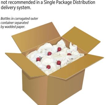
Paper dunnage can compress under internal movement of contents and allow glass containers to become unstable.
