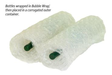
Bubble Wrap<sup>°</sup> cushioning requires a minimum of 2" of material around sides, top and bottom of bottles. Special attention must be paid to lock Bubble Wrap<sup>°</sup> securely to contents and add extra void fill when necessary.
