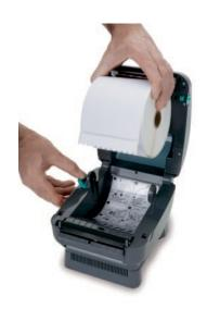
4. Make sure that the core is resting on the hangers and that the roll turns freely.
